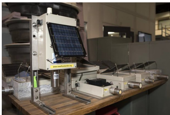
Figure 2. Several bridge sensors being constructed and prepped for deployment.
