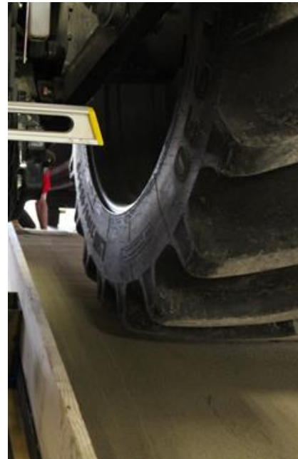
Row-Crop Tractor 4,790 lbs/per (480/80R50)@26PSI, rut depth = 5.5 cm (2.17 in.)
